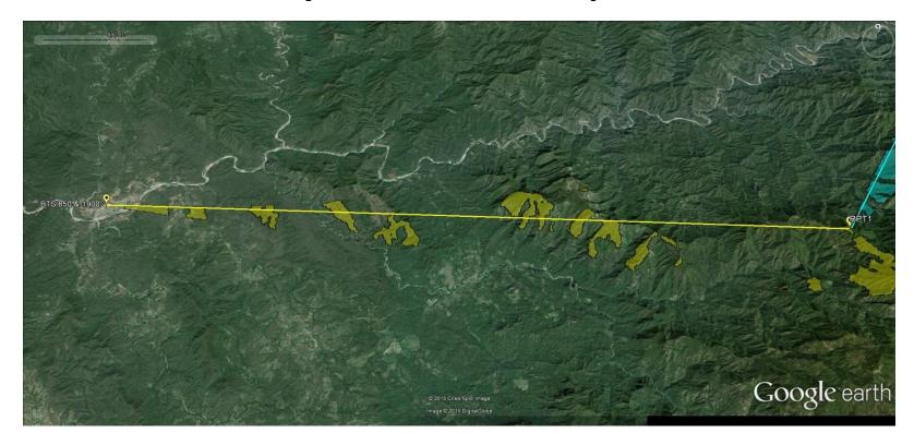
Example of first Repeater Link proving coverage to RPT1 location
