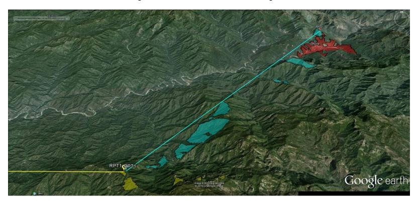
Example of second Repeater Link proving coverage to RPT2 location
