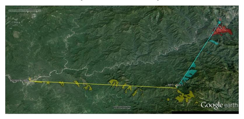
Example of 65 Km Dual Repeater Link proving coverage to main office and ATMs
